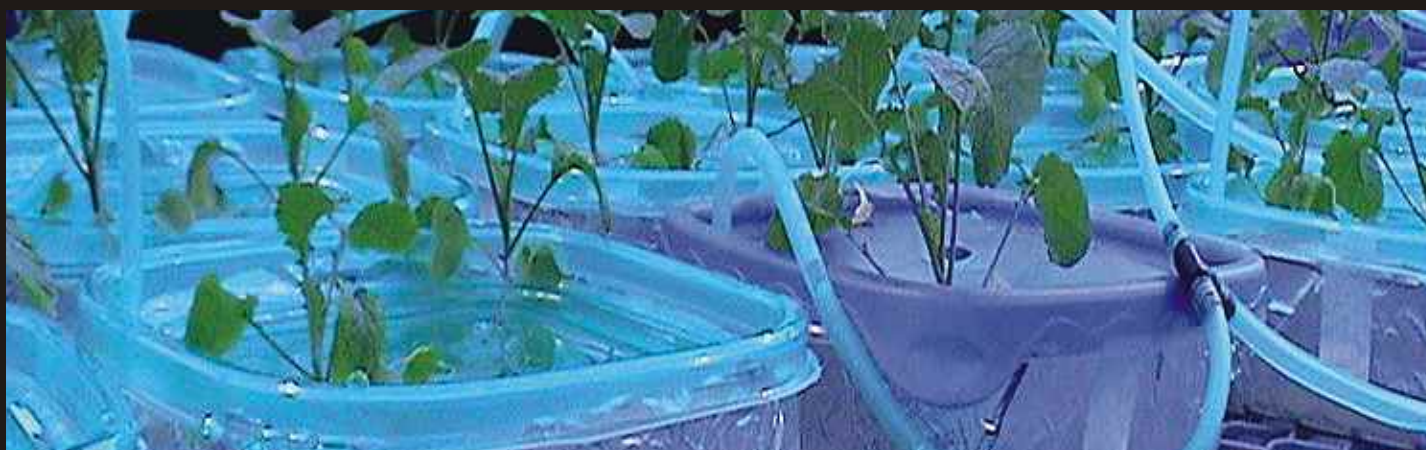
Hydroponics experimental setup showing Brassica juncea for removal of nitrate from wastewater
